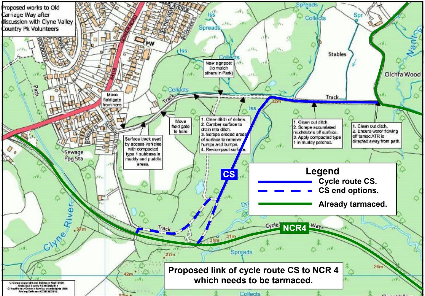
The base for the above map was prepared by Swansea Council to show their plans to upgrade the Old Carriageway Drive. The blue lines have been added to show the west end of Wheelrights cycle route CS (part of which includes ATNM route SWA75). CS is shown on Wheelrights SW Swansea map on the Routes page of their website: <https://www.wheelrights.org.uk/SwanseaCRsw.pdf>. CS needs to be surfaced to make it suitable for cyclists. A horse-friendly form of tarmac is suggested.
