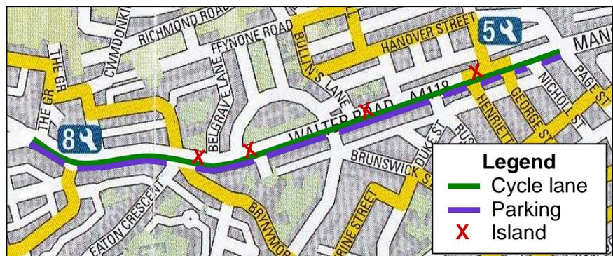
We noted that if parking was provided on the same side as a cycle lane (as shown on the plan above) a buffer between the footway and the cycle lane would be needed to safeguard cyclists from 'dooring'. (A buffer is shown on the Council drawing for the single lane option.)
